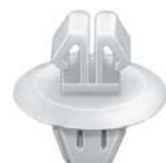
22456 (Toyota: 62955-50010) Yellow Nylon Rocker & Quarter Vent Moulding Clip with Sealer Top Head Size: 8mm x 8mm Bottom Head Diameter: 15mm Stem Diameter: 8mm x 8mm Stem Length: 11mm Lexus ES 250, HS 250h, LS 460, LS 600h L, RX 350 & RX 450h and Toyota Highlander, RAV4 & Yaris 2013 - On
