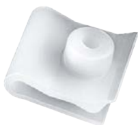
21017 (76882-0M000) White Nylon Nylon U-Nut Screw Size: M4.8 (#10) Panel Range: Up to 1.5mm Center of Hole to Edge: 8mm Nissan & Infiniti 1995 - On
