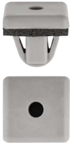
22297 (87759-3S000) Gray Nylon Rocker & Exterior Trim Moulding Grommet with Sealer Screw Size: M4.2 (#8) Head Size: 16.5mm x 16.5mm Stem Diameter: 12.5mm Stem Length: 12mm Overall Height: 15mm Hyundai Azera & Sonata 2011 - On
