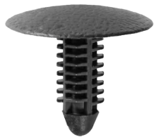
23745 Charcoal Nylon Trim Panel Retainer Head Diameter: 1" Stem Diameter: 5/16" Stem Length: 25/32" Panel Range: 0.080-0.532"
