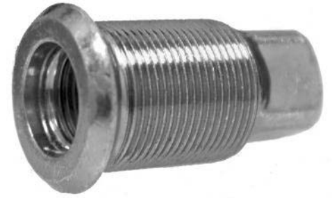
1-1/8" Inner Cap Nuts 3/4"-16 Inner Thread; 1-1/8"-16 Outer Thread Zinc Plated
