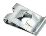
13225 Plated U-Type Nut Screw Size: 4.2mm (#8) Width: 11mm Length: 16.5mm Panel Range: .5mm-2.5mm Center of Hole to Edge: 8mm
