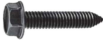
17035 (384931-S36) Yellow Zinc Dichromate 5/16"-18 x 1-1/16" Hex Head Sems® with Dog Point Washer O.D.: 7/8" Hex: 1/2" Ford
