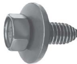
11109 (3986997, 14011722) Phosphate 3/8"-16 x 1" Hex Head Sems® Washer O.D.: 1" Hex: 9/16" GM
