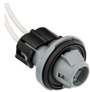
23127 (12141388, 88986416, LS44) Backup, License Plate, Side Marker, Parking & Turn Signal Lamp Socket Assembly Gauge: 20 Two TXL 8" Leads For T-3-1/4 Wedge Base Bulbs GM Cars & Trucks 1992 - On, Isuzu Hombre 1996 - On
