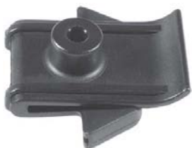
19735 (63848-5HA0A) Black Nylon Fender Clip U-Nut Screw Size: M4.8 (#10) Width: 20mm Length: 32mm Panel Range: Up to 2mm Center of Hole to Edge: 8mm Maxima & 240SX 1994 - On
