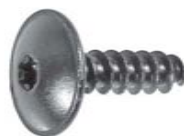
21541 (13144822) Black Zinc M5.5 x 20mm (12 x 25/32") Torx® Truss Head T-20 Drive Head Outer Diameter: 15mm (19/32") Use with Auveco 21539 & 21540 GM 2011 - On; Saab 2003 - On UNIT PACKAGE: 25
