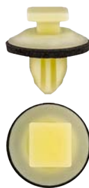
22456 (Toyota: 62955-50010) Yellow Nylon Rocker & Quarter Vent Moulding Clip with Sealer Top Head Size: 8mm x 8mm Bottom Head Diameter: 15mm Stem Diameter: 8mm x 8mm Stem Length: 11mm Lexus ES 250, HS 250h, LS 460, LS 600h L, RX 350 & RX 450h and Toyota Highlander, RAV4 & Yaris 2013 - On
